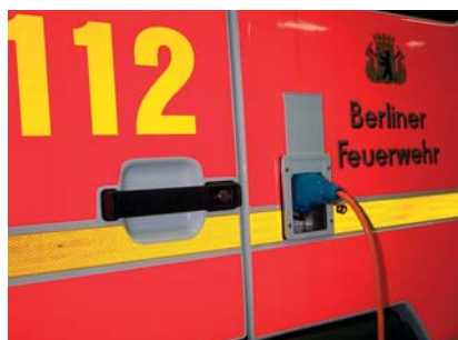
Enclosure fitted with control light (LED)
