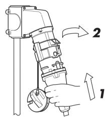
To connect the plug, align its bayonets and the hollow parts of the socket-outlet, push the plug partially, locking finger facing upward, and turn it clockwise as an electric light bulb.
