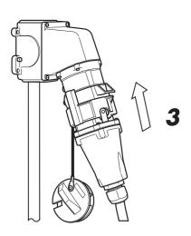
In absence of a lock-out, the circuit is finally closed by pushing the plug fully home until it is held by the locking ring. The window located on the front of the socket-outlet becomes «red». IP67 is achieved by turning the ring clockwise. If the knock-out hole has been opened, the plug can be padlocked into the socket-outlet.
