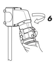
To remove, twist and withdraw the plug. The lid must then be shut and the ring turned to restore IP67 of the socket-outlet.
