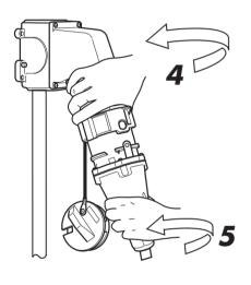
To release the plug, simply turn the ring fully anticlockwise. The circuit is open (green indicator) and the plug is in its parked position.
