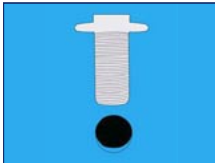
Clearance hole = Thread diameter + 2mm max.
