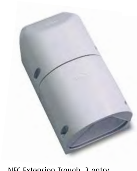
NEC Extension Trough, 3 entry Created by coupling NEA trough to NEB Terminals can be installed in either upper chamber (NEA) or lower chamber (NEB) Height 180mm, Width 98mm, Depth 93mm
