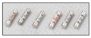
Lawson Type "PL" fuse-links are intended primarily for use in domestic plugs but may also be installed in appropriate single-phase installations with fault levels up to 6kA and have nominal dimensions of 6.3 x 25.4mm.
