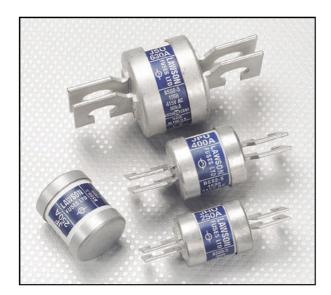
The range has a rated voltage of 415V a.c. and has been certified at a test recovery voltage of 110%. These fuse-links are therefore suitable for use on systems with voltages up to 457V a.c. The rated and test voltages also ensure that the range meet all the transitional voltage requirements specified within the harmonised nominal voltage of 400V a.c.
