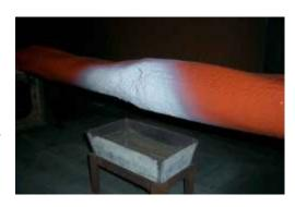
The system incorporates a flexible outer fire barrier tube that provides a high degree of fire resistance. For installations outside of the tunnels this can be omitted.
