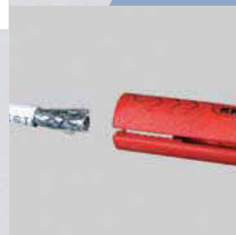
Dismantling a Coax-cable 4.8 – 7.5 mm Ø
