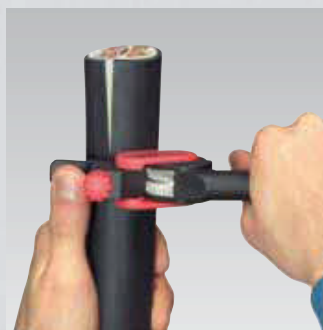
Turning the tool for circular cut
