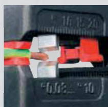
Precise stripping prevents damage to the conductor
