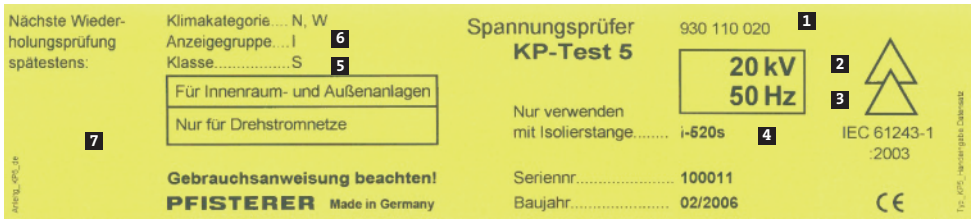
Figure 3: Voltage tester nameplate (example) and explanations
