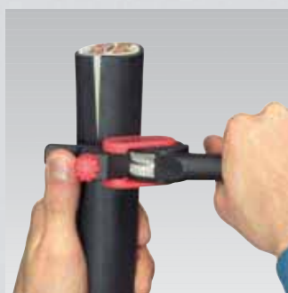
Turning the tool for circular cut
