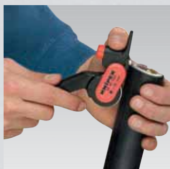
Setting the tool for longitudinal cut
