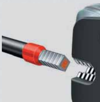
Square crimping for optimum contact zones
