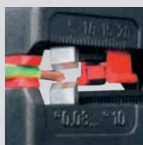
Precise stripping prevents damage to the conductor
