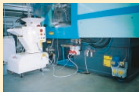
Plastics moulding department. Injection press equipped with TER series interlocked socket-outlets.
