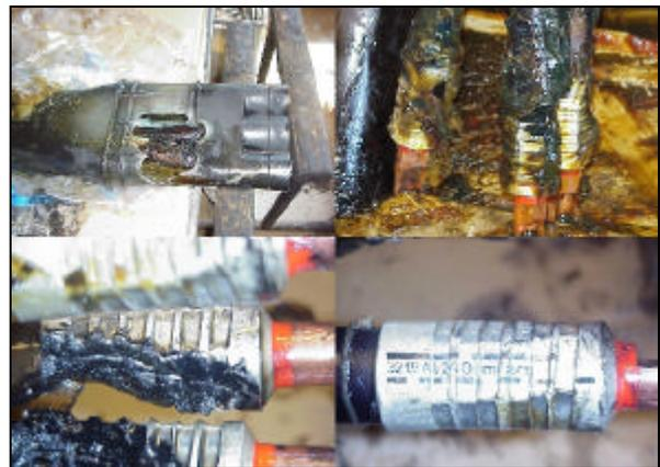
**Figure C1:** *Fault cause analysis of disturbed cable termination. Several sharp edges on the connector were found on all three phases.*
