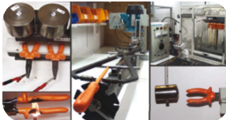
Laboratory equipped with control means allowing guarantee the conformity with CEI900/EN60900/ASTMF 1505-94 standards.
