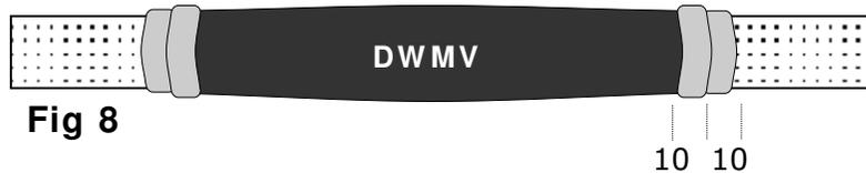
10. Apply the pieces of grey mastic tape (4SC HV) to the connector insulation tube ends as shown in Fig 8. Overlap on to the DWMV tube and paper screen insulation by 10mm either way.
