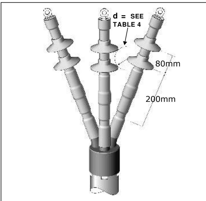
The first shed should be fitted at a distance 200mm from the lower edge of the anti-track tube to the edge of the shed. All subsequent sheds should be fitted at a distance of 80mm from edge to edge.
