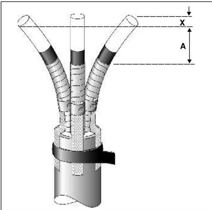
Remove the copper tape screen to length  $A+X$  as indicated in Table 2.
