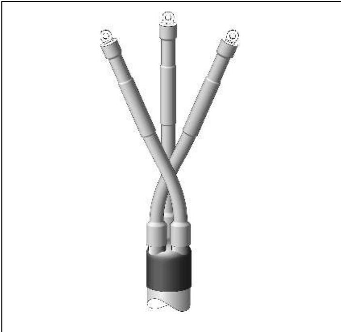
If it is necessary to cross the cores, the cross **MUST** be in a screened area as shown.
