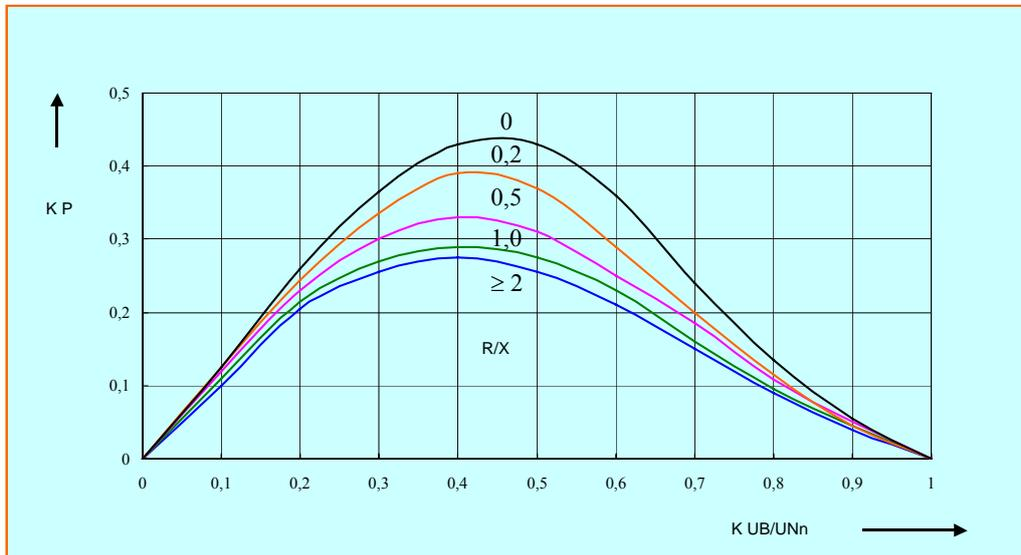
Figure. 1: Factor  $k_p$  for determination of arc power [3]
