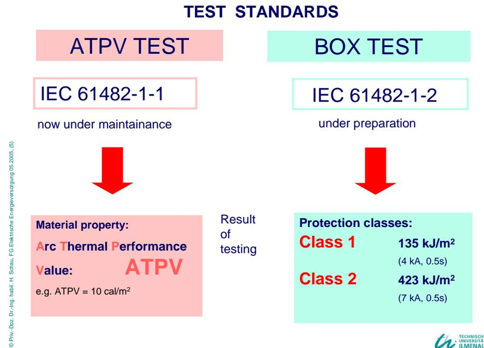
Figure 3: Future test standards within IEC 61482
