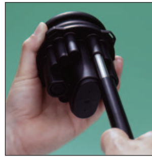
(1) Punch out base hole with port tool
