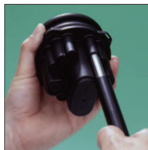
(1) Punch out base hole with port tool
