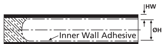
b: Fully recovered form (after heating)
