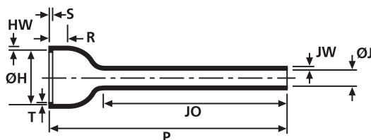
b: Fully recovered form (after heating)
