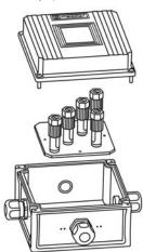
Do not over-tighten the self-tapping screws supplied with polymeric accessories.
