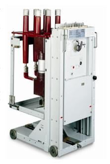
We can supply a type tested vacuum circuit breaker as a direct retrofit for the oil circuit breakers in the VSI and VTD switchgear. This vacuum circuit breaker has more than two decades of reliable and proven operational service experience throughout the world in the Hawker Siddeley Switchgear Ltd VMV range. Only very minor modifications are required to the existing switchgear fixed portion.
