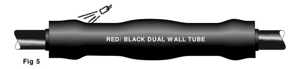
4. Position the stress control and red/black dual wall tubes over each core.
