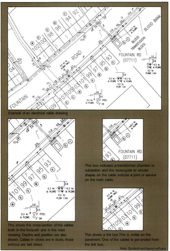
Figure 7 Example of an electricity plan
