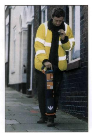
Figure 4 Using a cable locator
