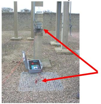
Maximum of 0.025 Ohms between the mat and the handle mechanism box
