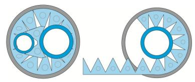
The unique design of the tri-flexible foam makes positioning and separation of the cables very simple while also providing a backing for the MD+ to be applied on.
