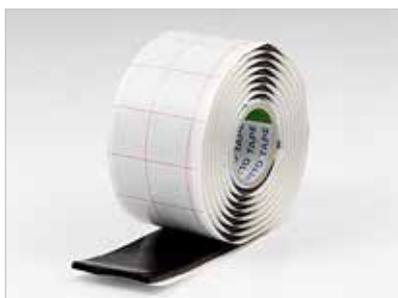
Nitto 12FB is a self amalgamating putty tape. By stretching and wrapping around pipefittings, cables, or other objects, the putty will instantly amalgamate into itself, thus creating a waterproof barrier to prevent corrosion. 12 FB is suitable for in and outdoors.
