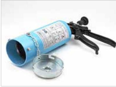
Filoform injection pumps are used to pump the resin under pressure ( $\pm 2$  Bar) into injection joints. The injection pump has a continuously variable piston displacement enabling an optimal flow of the resin into the joint. The injection pump type 710ml has a larger capacity than the injection pump type CN-E4 (355ml) and is therefore suitable for all resin bags to 710ml.
