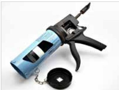
Filoform injection pumps are used to pump the resin under pressure ( $\pm 2$  Bar) into injection joints. The injection pump has a continuously variable piston displacement enabling an optimal flow of the resin into the joint. The ball bearing mechanism reduces the manual effort required to fill the joint.
