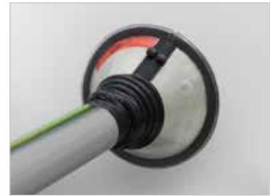
Duct sealing system type MDII has been developed to provide an effective and simple solution to all gas- and watertight duct sealing requirements. MDII will not only seal the space between the cable or pipe but also the space between the duct and the wall in one operation.
