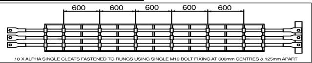
The example shown relates to BS EN 50368:2003 tests only. Other configurations / cleat spacings can be accommodated dependant on the fault level applicable. Please refer to Ellis Patents for further information.
