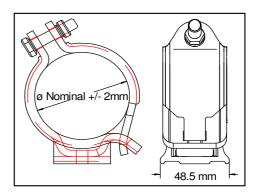
Maximum and minimum cable diameter nominal ± 2mm
