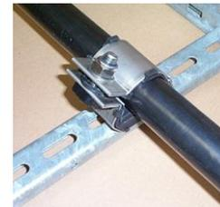
Please note: Thread galling is a known phenomenon which can occur when using stainless steel fasteners. A breakdown in the material's protective oxide layer results in the set screw and nut becoming welded together. To reduce the incidence of thread galling excessive pressure and speed should be avoided during installation. Thread lubricants can also be used at the point of application if problems are experienced - please contact Ellis Patents for further information.
