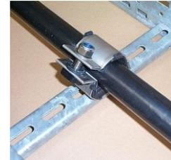
5) **Important.** Do not over tighten the cleat. The liner should be in contact with the cable but does not need to be so tight that the cable bulges at either side of the liner.
