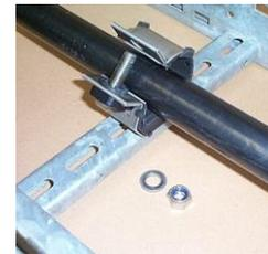
4) Close the hinged arm and refit the washer and nyloc nut (19mm socket required). The head of the screw is held in position so that only a single power tool is required to tighten the nut from one side.
