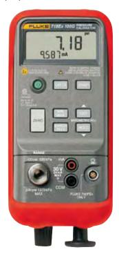
The 718Ex is a powerful intrinsically-safe, self contained pressure calibrator for usage in ex-hazardous areas. The calibrator offers:
