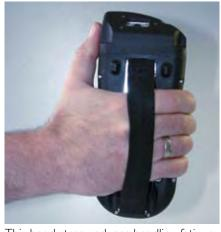
This hand strap reduces handling fatigue and helps prevent accidental dropping.
