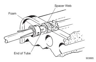
3.07 Mix one bag of sealant foam according to the instructions on the bag.
