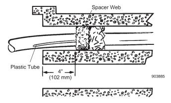
3.05 Wrap foam strip around cable and insert it into duct. The foam strip should be flush with the duct entrance and should fit snugly between the cable and duct.
