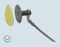
With terminal thread M16 for higher current loadings (50 Hz), e.g. for connection of the ring equipotential bonding at the earth-termination systems of power systems with nominal a.c. voltages exceeding 1 kV (transformer earthing).
