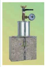
Figure 2: Set-up for the pressure water test
