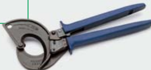
KT 4 For cutting cables Ø max 52 mm Weight: 0,89 kg Length: 310 mm
