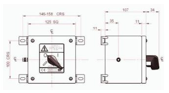
Mounting Holes - M6 Termination - M4 Maximum Cable Size - 6 mm<sup>2</sup>
