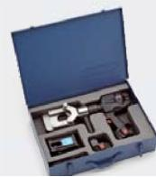
14.4 V cordless hydraulic cutting tool, lightweight and balanced for single hand operation. Specifically designed cut copper. aldrey, aluminium, aluminium-steel cables and steel ropes, aluminium and steel rods having a max overall diameter of 55 mm.
