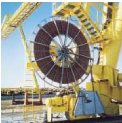
A Cavotec Specimas cable reel working at \pm 200 m/min on a P&H log-handling crane for Federal Paper Board, in Augusta USA.
