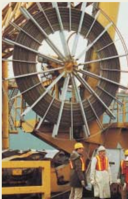
A large, high speed Cavotec Specimas cable reel mounted on a coil handler running at 180 m/minute.
