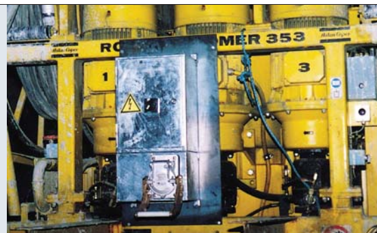
A Cavotec panel mounted on an Atlas Copco shotcrete machine.
