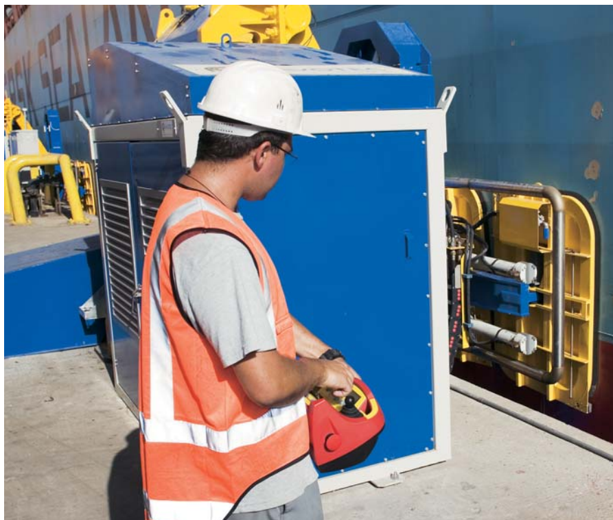
MC-3000 used together with a Cavotec MoorMaster unit to control the mooring operation, and also to monitor from the ship's bridge all alarms or incidents that take place.
