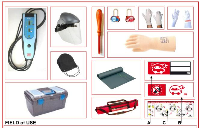
Equipment necessary to make the securing electrical operations on electrical vehicle. In accordance with UTE C 18-550 standard.
