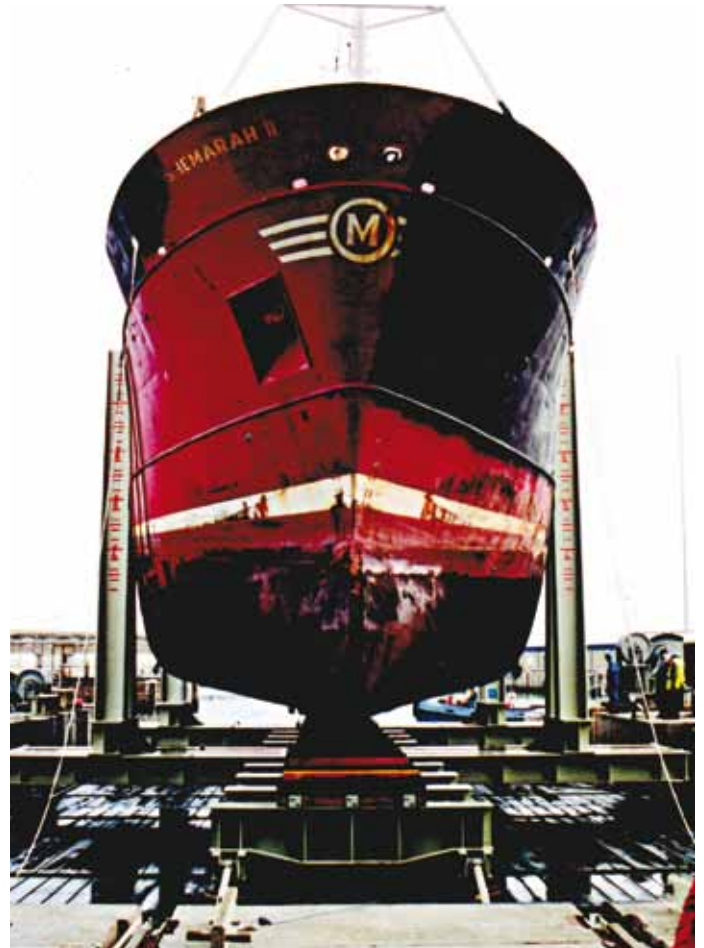
Syncrolift in operation at Peterhead Harbour.
