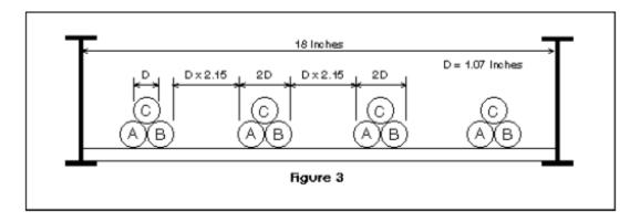
The installation of the cables in the cable tray as per Figure 3 is very desirable for the reasons stated concerning Figure 1A.
