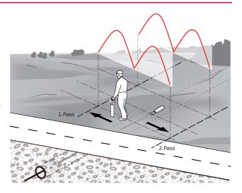
If a "walk through" sewer is being traced, another vertically, for example to pinpoint a buried manhole.
