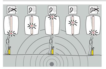
Move backwards and forwards over the service until the highest signal reading (peak response) is located. The service is directly below the EziCAT when the LED bar display is at its maximum reading. The EziCAT audio signal will automatically adjust to facilitate pinpointing over the service.
