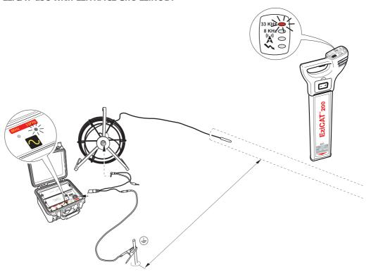
Connet the EziTRACE to the EziROD and also to earth stake as shown. Inserted and push the rod into the service to be traced. Set both EziTRACE and EziCAT to 33 kHz mode and use the EziCAT to trace the signal and therefore the service along the full length of the EziROD wire.
