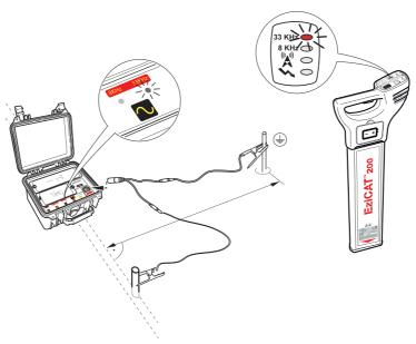
Attach the Clip on the red cable to the metallic service. Attach the clip on the black cable to earth stake positioned at right angles and as far as possible from the service to be traced. Set both EziTRACE and EziCAT to 33 kHz mode and use the EziCAT to trace the service. For details see "5 Tracing Modes Summary".
