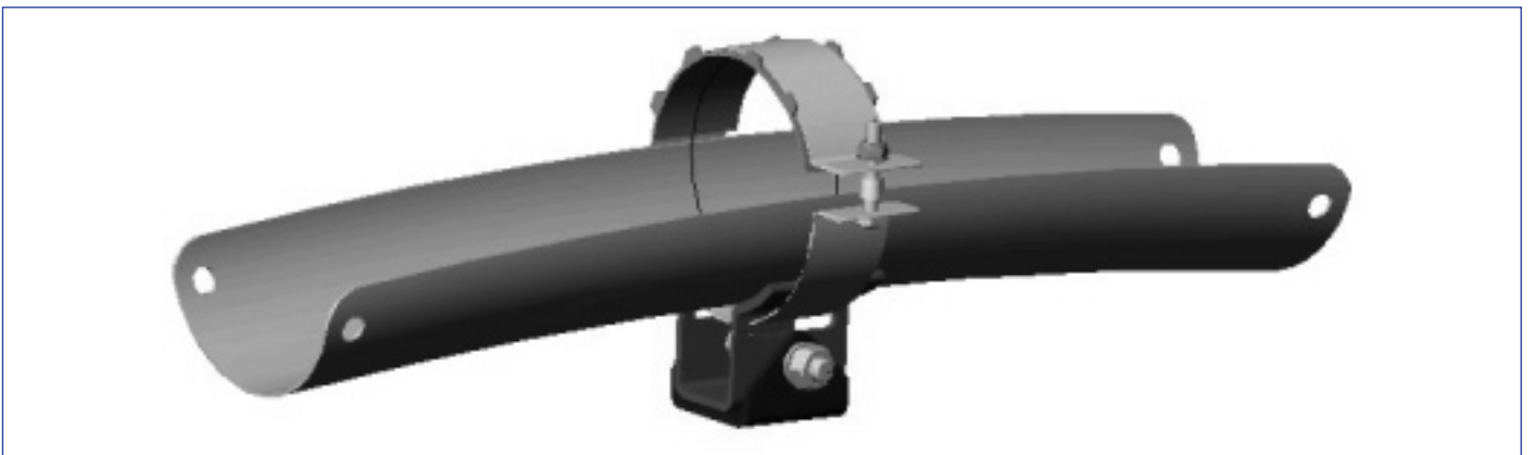
7. Cable cleat with combined support saddle for 150mm diameter cable fixed at 8.2m centres.
