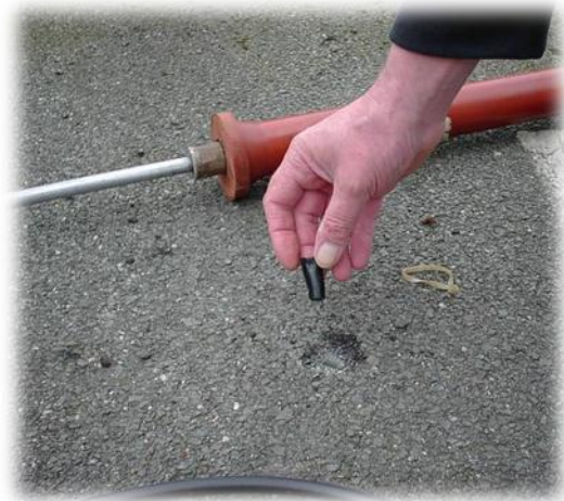
Repairing the hole with a Tar Plug
