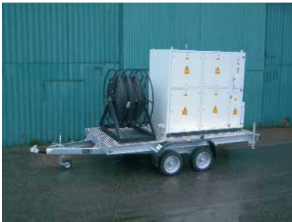
Turntable Steer Trailers - Model shown is 12000Kgs gross fitted with ABS braking to full UK highway specification
