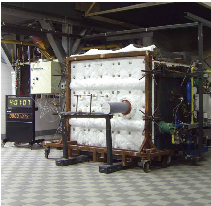
In-house fire testing and pressure testing at CSD International's Laboratories.
