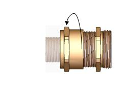
**3.** Locate the detachable armour cone (C) into the recess of sub-assembly "A". Pass cable through sub-assembly "A" evenly spacing the armour around the cone.
