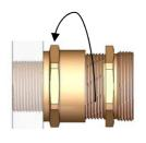
**6.** Hold the main item with a spanner, then re-tighten the sub-assembly "B" onto sub-assembly "A" ensuring the two components are fully tightened.
