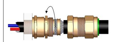
**2.** Locate the detachable armour cone (C) into the recess of sub-assembly "A". Pass cable through sub-assembly "A", evenly spacing the armour around the cone.
