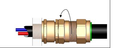
7. Tighten the outer seal nut until either:
