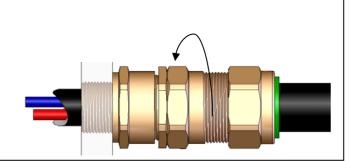
**6.** Tighten the outer seal nut until either:
