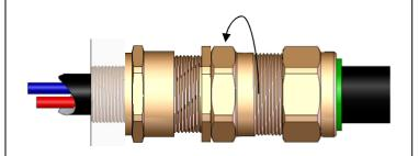
**5.** Pass cable through sub-assembly "A". Tighten the main item by hand until heavy resistance is achieved, then tighten a further full turn with a spanner.
