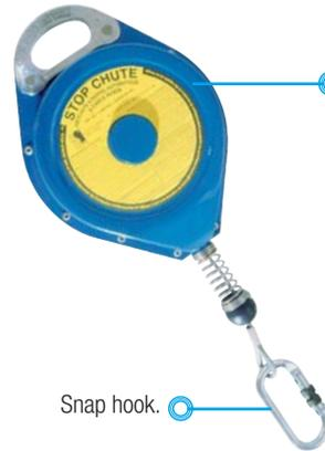
Integrated braking mechanism and dissipating element. Self locking mechanism and automatic tensioning and return facility.
