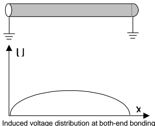
Induced voltage distribution at both-end bonding
