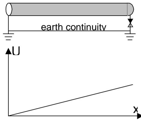
Induced voltage distribution at single-end bonding
