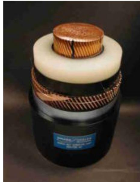
Typical sample of a 2500mm<sup>2</sup> 500 kV XLPE cable
