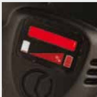
Battery condition display
