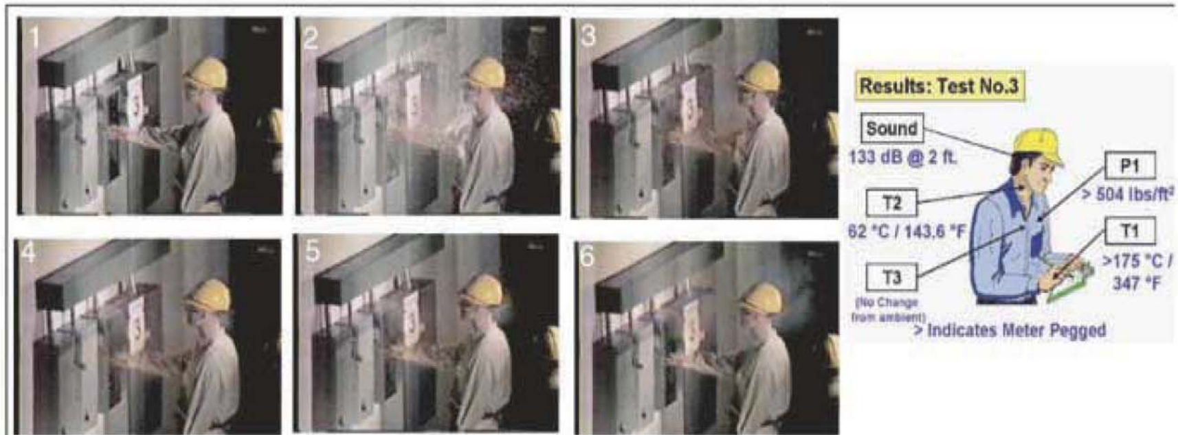
Figure 4. Test 3 - 22,600-A rms, 480-V, fault initiated on line lug of size 1 starter, feeder protected by a 601-A current-limiting device and fault was cleared in 1/2 cycle.
