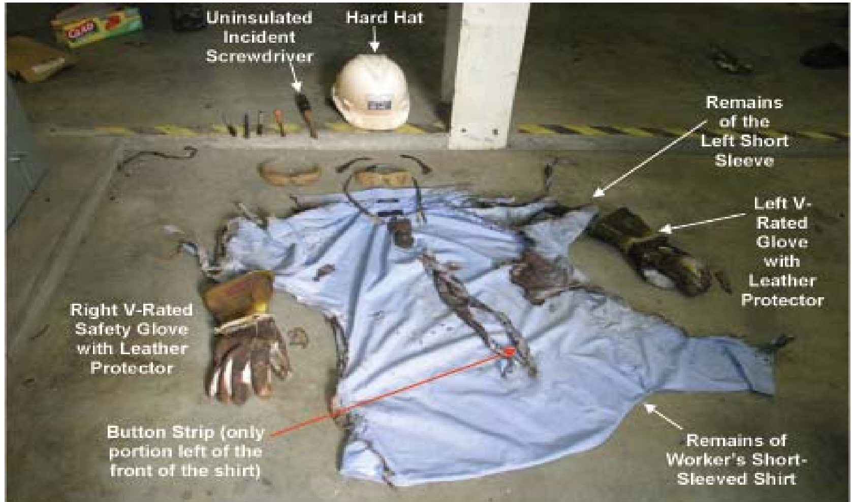
Figure 2-6. BSE-1's burned shirt and his flash-damaged PPE and tools
